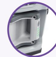
**Battery Fuel Gauge** indicates the approximate runtime remaining on the battery pack when the display button is pressed. 4 lights: 80%-100%; 3 lights: 60%-80%; 2 lights: 40%-60%; 1 light: 20%-40%; 1 flashing light: Less than 20%.
